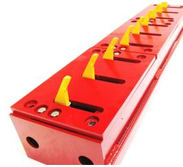
1. Install the Directional Traffic Controller perpendicular to the flow of traffic. If vehicles cross the controller at an angle other than 90 degrees the spikes may cause sidewall damage to the tires. Check all bolts to insure none have loosened during shipping, and tighten as necessary. Loctite is recommended for final installation.
